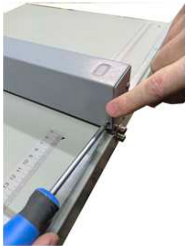
Again undo the screws on the other side of the cover
