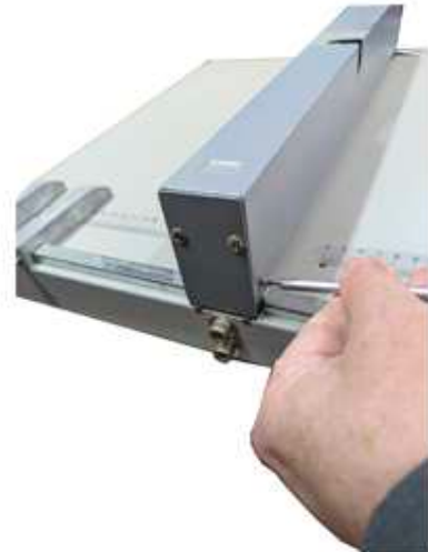
Undo the screws each end which hold the creasing bar cover
