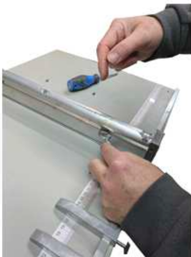
Use a spanner to turn the adjusters at each end of the bar - clockwise = lighter crease, anti-clockwise = deeper crease. Test a sheet of paper and keep adjusting until you are happy and the bar is level
