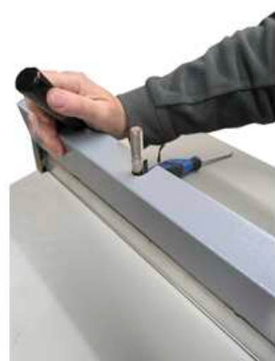
Once adjusted, re-attached the cover, do up the cover screws and re-attach the black handle. Some thicker card may require more adjustments for a good crease as they vary in resistance
